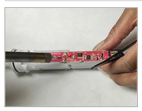
De-Solder the three (3) upper terminals from the circuit board.
