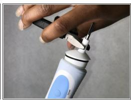
Pull off head, and use pliers to remove the white cap. Pull out the circuit core.
