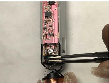
De-Solder lower battery connection terminal. Bend back battery terminal to clear circuit board.
