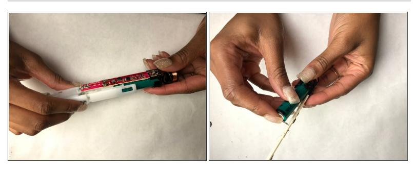
Pull the circuit board and battery assembly out. Then proceed to remove the battery from the circuit board
