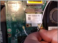
• Remove the white and the black antenna wires from the wifi module.
