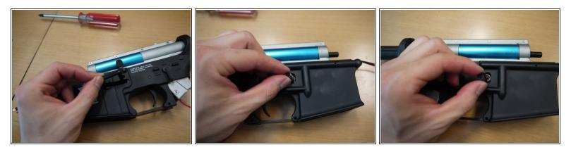
• Reinstall the mag catch, then place the spring on the post and the button on top of it. Tighten the screw that holds the button in place.
