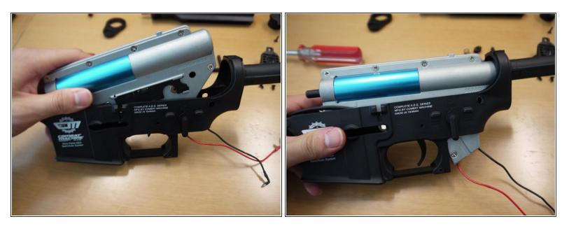
• Make sure that the selector is set to semi-auto, and place the gearbox back into the lower receiver.
