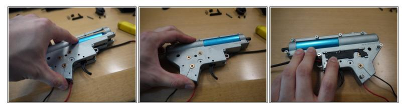
• Ensure that the gearbox is fully closed before reinstalling the screws. Forcing the screws in while the gearbox has misaligned parts will damage the gearbox.
