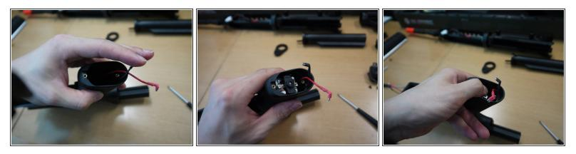
• Arrange the wires so that both are against the rear of the pistol grip. Place the motor in the pistol grip, making sure that it slides in freely and bounces back from spring tension after you push down on it.
