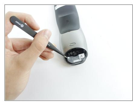
Using tweezers, peel off the sticker located under the battery cover to reveal two screws.
