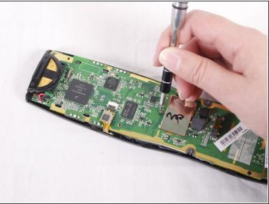
• Using the Philips #0 screwdriver, remove the three 50mm screws from the circuit board.
