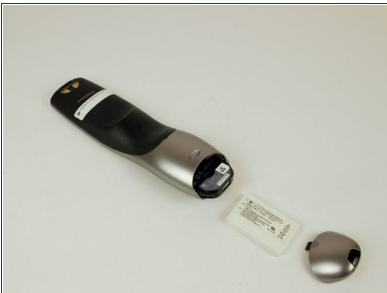
Push the battery in, pull it up, and slide it out.
