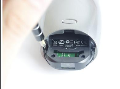
• Locate and unscrew the four 50mm screws using the Philips #0 screwdriver.
