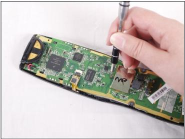
Using the Philips #0 screwdriver, remove the three 50mm screws from the circuit board.
