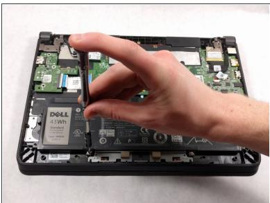
Using a JIS #0 screwdriver, unscrew the two 4mm screws securing the battery in place.
