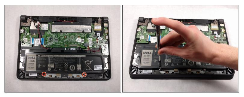
• Using a JIS #0 screwdriver, unscrew the two 4mm screws securing the battery in place.
