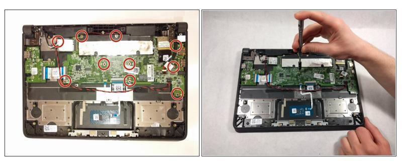
Using a JIS #0 screwdriver, unscrew the ten 4mm screws securing the motherboard in place.
