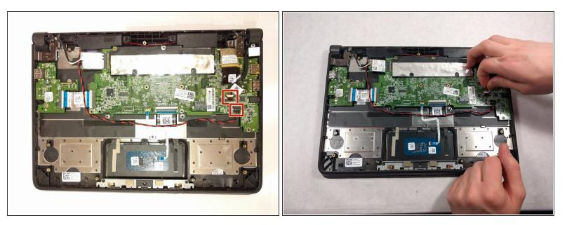
Remove the two 4-pin connectors that are also connected from other components in the device.
