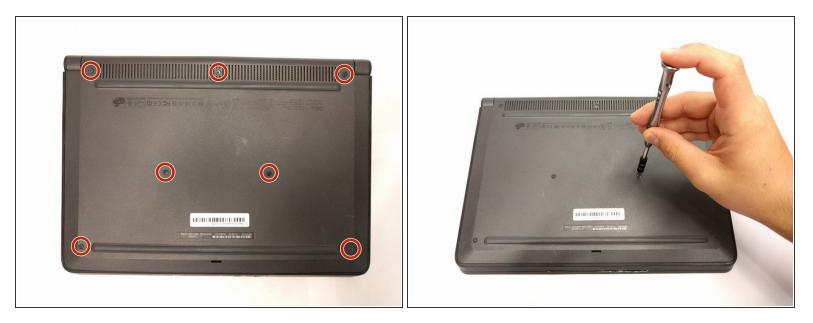
Use the #J0 screwdriver to unscrew the seven 4mm screws located around the back panel.
