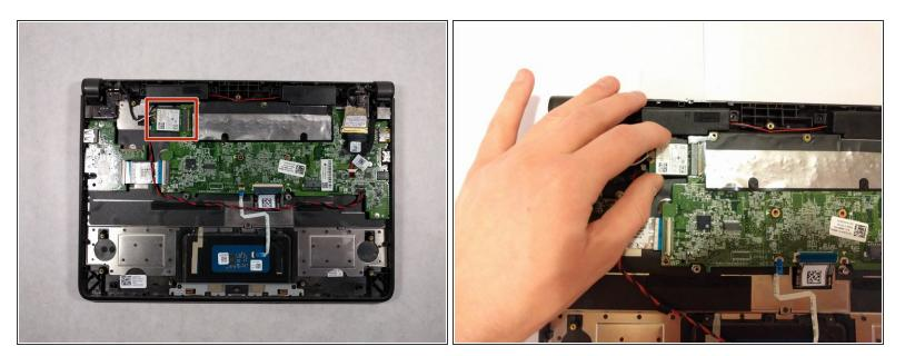
Disconnect the small chip that connects to the motherboard by gently tugging on it in the direction away from the board.
