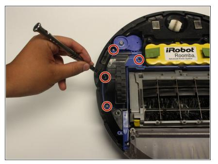
Remove the 15 mm screws with the Phillips #0 screwdriver bit.
