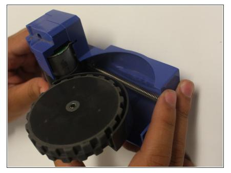
Once the screws have been taken care of, the wheel component (with the spring inside) can be removed from the main assembly.
