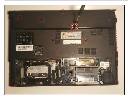
Remove the eleven screws that hold that back panel to the laptop using a J0 Phillips screwdriver bit.
