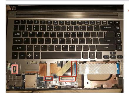
• Next, disconnect the 4 wired tapes of the keyboard from the motherboard just like we did with the lower front touchpad panel.
