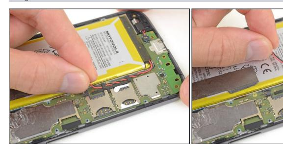
• Peel off any tape securing the battery wires, and then push the battery wires towards the battery to de-route them from the black bracket on the motherboard.
